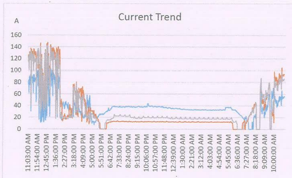
Figure6. Main Incomer Current Profile
